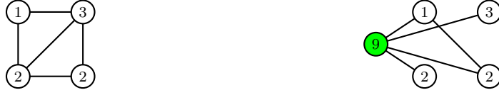
FIGURE 4.1. The approximation preserving reduction from K_3 hitting set to CLAW-VD. On left is the K_3 hitting set instance G, w . On the right we take the complement and add green apex with more than the total weight G', w' .
